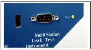
The setup and operation commands for communications to and from the Sentinel M24 are accessed via the INSTR CONFIG key. For serial communication, the operator must select either RS232 or IrDA. The Sentinel M24 instrument can only communicate via one of these two methods at a time. There is a nine-pin RS232 connection and an IrDA port on the front of the instrument, shown above There is also a five-terminal connector for RS232 on the internal I/O co-processor board, shown below.
