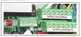
RS485 and TCP/IP communication can operate simultaneously with the serial communication of RS232 or IrDA. The RS485 and TCP/IP connections are internal to the instrument on the left side of the bottom board, shown below
