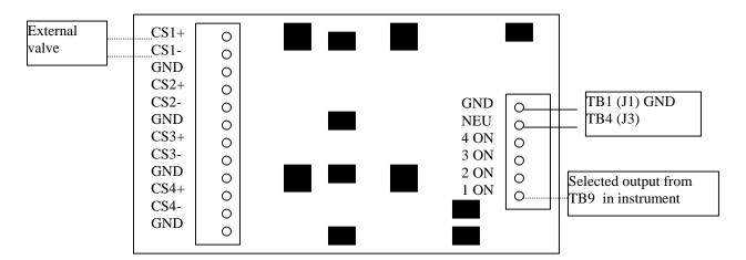
One coil saver board can convert up to four distinct inputs into pulse modulated outputs. 1 ON converts to CS1 (+ and -), 2 ON converts to CS2 (+ and 1), 3 ON converts to CS3 (+ and-), and 4 ON converts to CS4 (+ and -).
