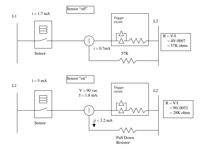
Note that this particular sensor has a "minimum load current" requirement, so we are obligated to use as 28K or smaller resistor. To be safe, we would choose a 20K resistor, which would have to dissipate  $(120)^2/20,000 = 0.72$  Watts. A 1 Watt resistor will get very hot dissipating this much heat. You need to plan accordingly.
